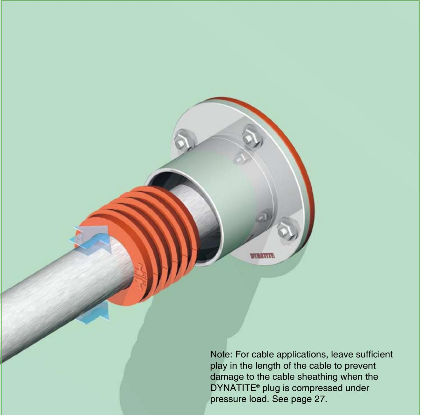
7) Both segments of the DYNATITE® sealing plug are placed around the ducted pipe/ cable, then pushed into the conduit sleeve as far as the first serration. The first serration is smaller than the other serrations to make this procedure very easy. Both halves are then pushed by hand evenly, further into the DYNATITE® conduit sleeve. The inlet of the DYNATITE® conduit sleeve is rounded off to avoid any damages to the plug during insertion.
