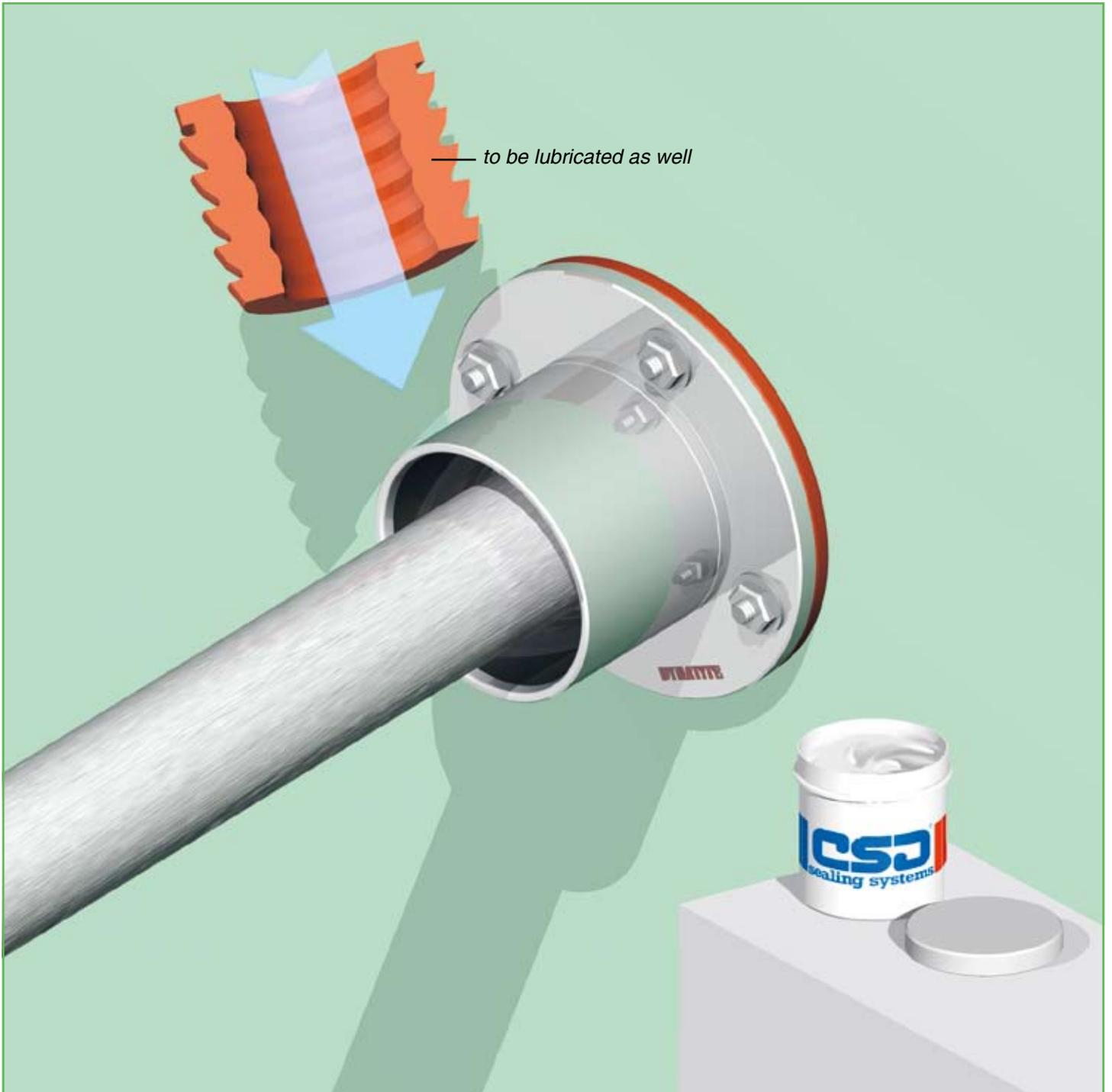
5) The inside surfaces of both segments of the DYNATITE® sealing plug are then lubricated with CSD® lubricant. Also the flat contact surfaces of the plug halves should be lubricated to enable equal insertion in the conduit sleeve. CSD® lubricant is acid free.
