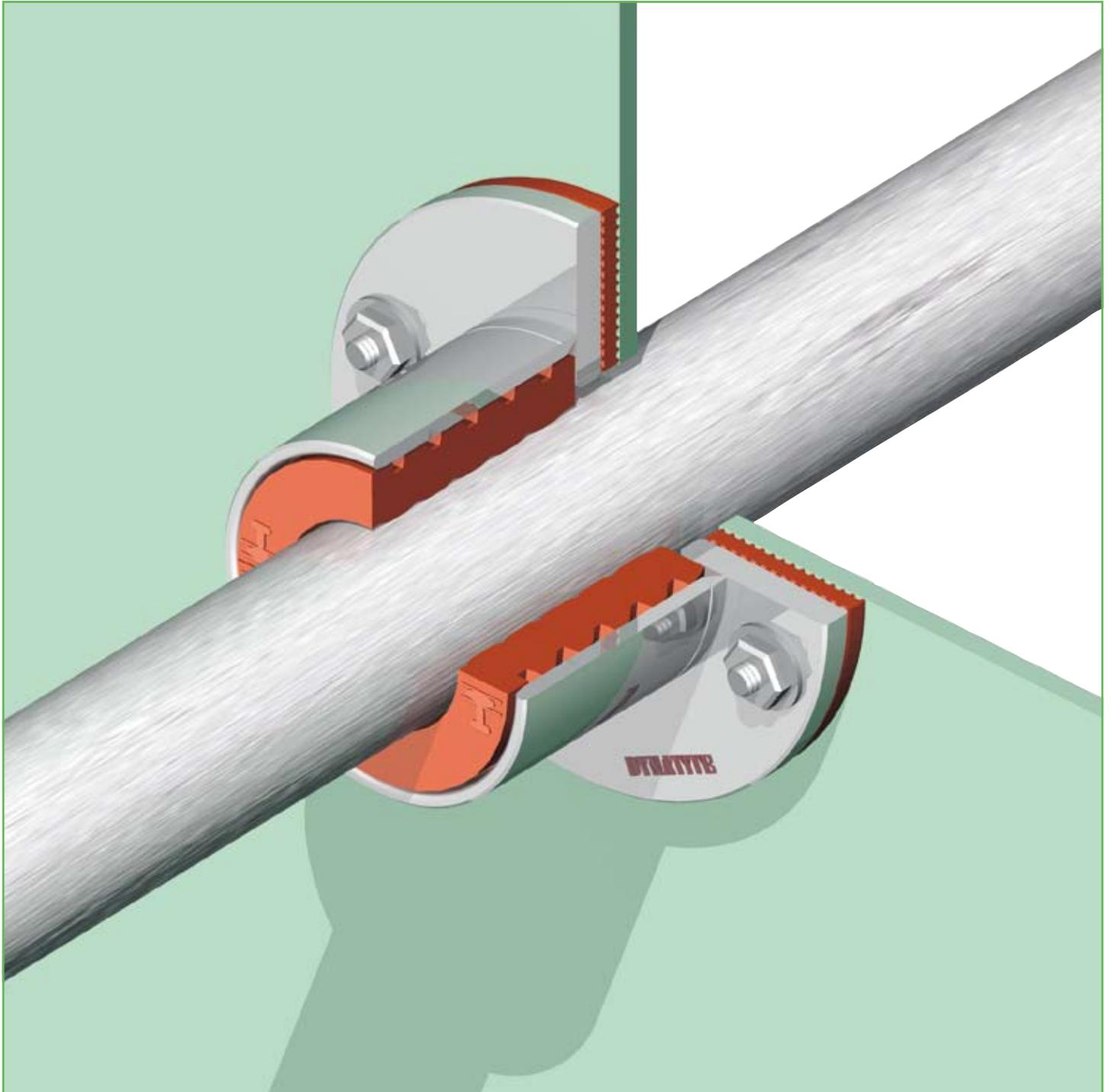
For existing installations, DYNATITE® conduit sleeves, which can be bolted to the partition, are supplied. These conduit sleeves can also be used to concrete walls in onshore installations. Since the conduit sleeves are ready for use and therefore don't have to be exposed to any welding heat, the inside of the conduit sleeve could be treated with a PTFE coating to improve the gliding properties even more compared to the ceramic coated welding sleeves.
