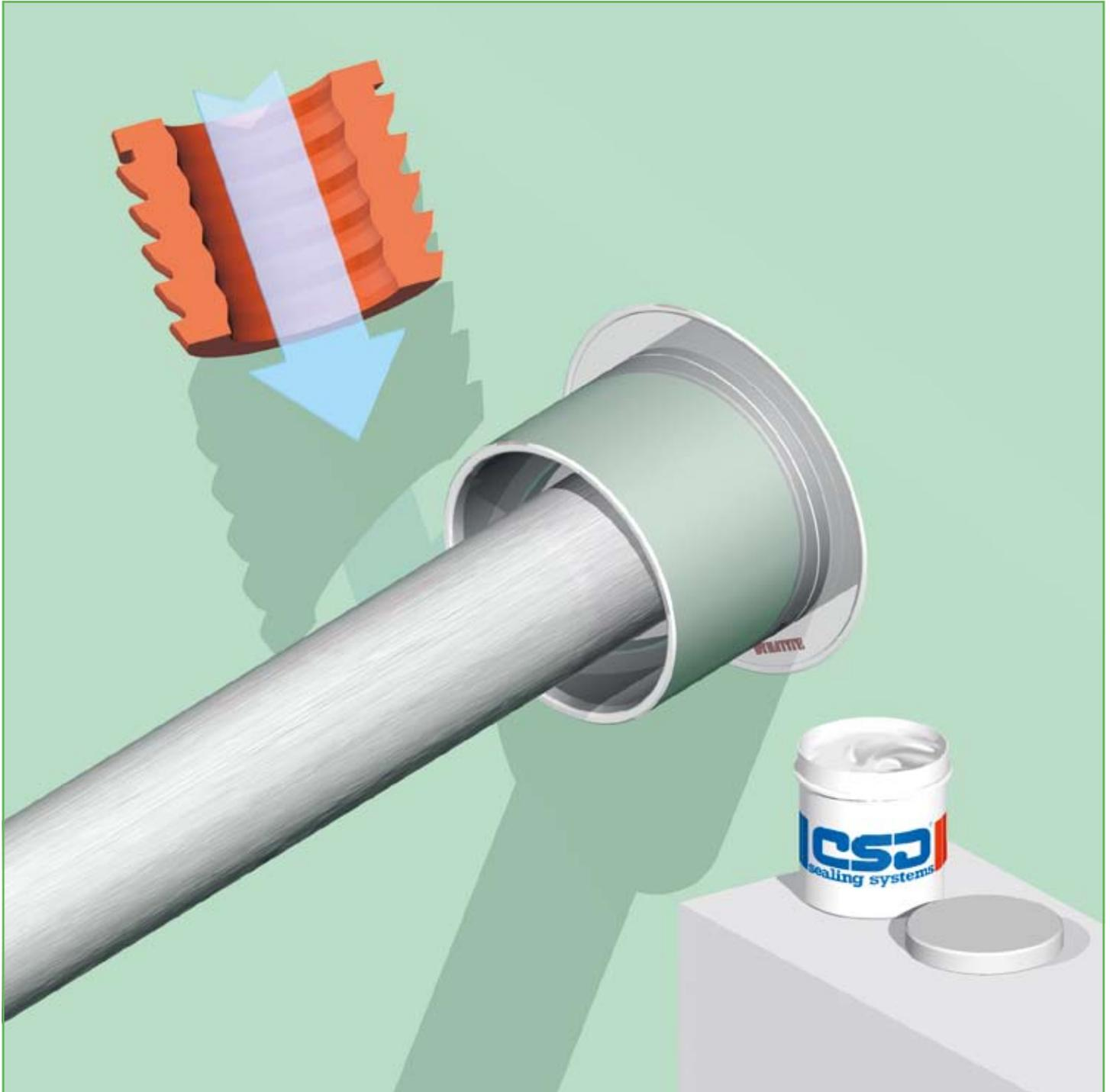
3) The inside surfaces of both segments of the DYNATITE® sealing plug are then lubricated with CSD® lubricant. Also the flat contact surfaces of the plug halves should be lubricated to enable equal insertion in the conduit sleeve. CSD® lubricant is acid free.
