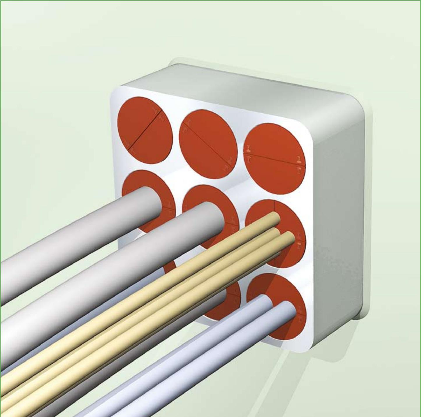
DYNATITE® multi-passage units which are manufactured with exact fitting dimensions to adopt the sealing plugs and to allow the required movement of the rubber. In this simple way, pressures in excess of 10 bar can easily be coped with. The DYNATITE® dynamic sealing system holds also static tight after dynamic exposure.
