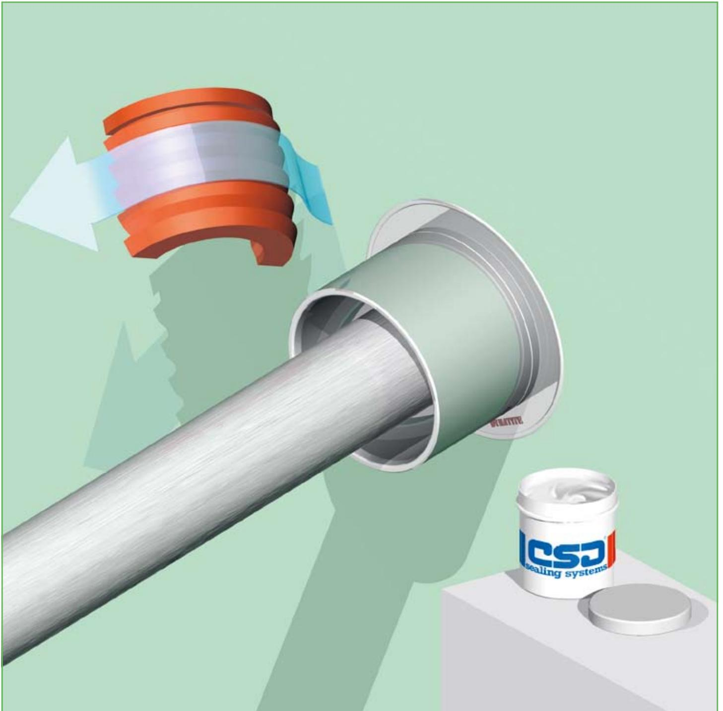
4) The segments of the DYNATITE® sealing plug are also treated with CSD® lubricant on the outside. Please refer to the Safety Data Sheet of the CSD® lubricant for more information.
