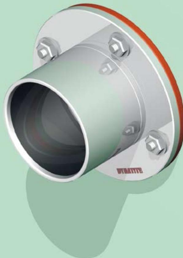
3) The DYNATITE® conduit sleeve can then be positioned and fixed to the partition. Avoid excessive forces on tightening to maintain the flexibility of the NOFIRNO® gasket and to guarantee tightness on long term.
