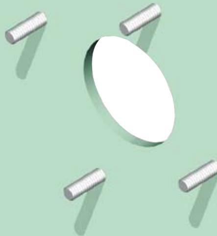
1) When DYNATITE® conduit sleeves for bolting are going to be used, a hole has to be cut in the partition to the size of the opening in the retainer flange of the DYNATITE® conduit sleeve. Threaded ends have to be welded to the partition in accordance with the hole configuration of the flange of the conduit sleeve. In case of application against concrete walls, stainless steel anchor bolts should be used.
