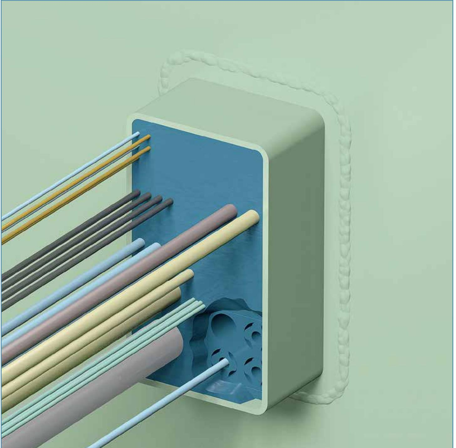
An open passage is now available for ducting a new cable through the existing CONTROFIL® multi-cable transit.
