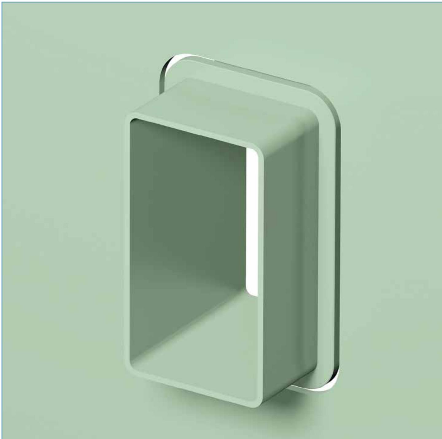
The welding flange is 10 mm thick, 15 mm high with rounded corners to enable good positioning for welding and to prevent welding stresses in the construction. The thickness of the welding flange prevents tilting of the conduit frame or destroying the thinner wall conduit frames during welding. The stainless steel CONTROFIL® conduit frames (1.4571) are passivated and are exposed in the technical laboratory of BEELE Engineering to a salt fog test for 20 years sea water resistance.
