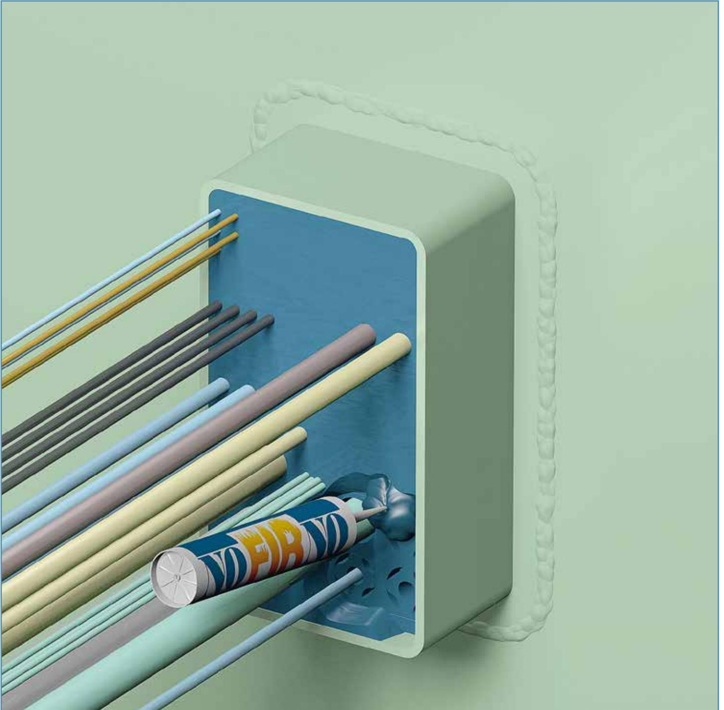
Clean and dry the wall of the transit frame inside as well as the newly ducted cables thoroughly and refill the opening in the sealant layer at both sides of the transit with NOFIRNO® sealant. The fresh sealant adheres very well to the already cured sealant. Finish the new sealant layer in the same way as done for the initial sealant layer.
