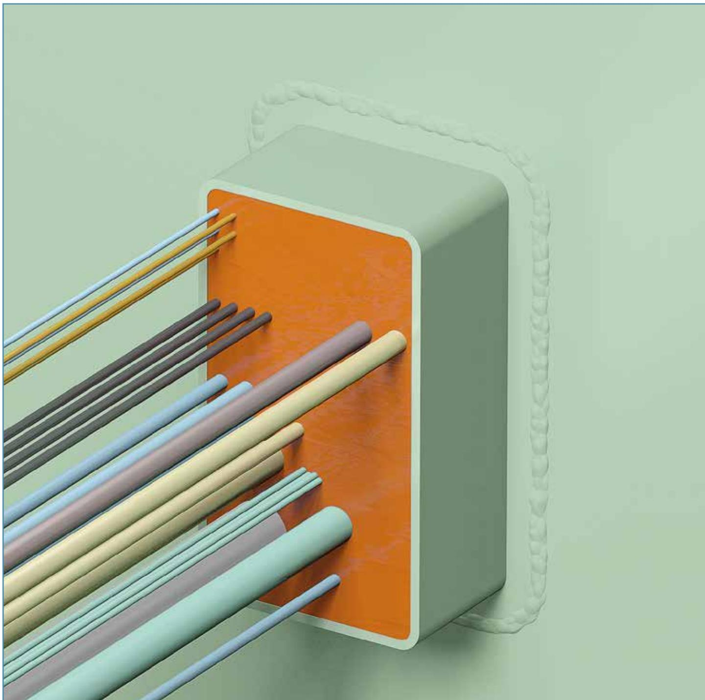
The CONTROFIL® block type multi-cable transit finished with the terracotta NOFIRNO® sealant. The CONTROFIL® multi-cable transits are very good UV, Ozone and weathering resistant. No metal parts are incorporated in the sealing system. No corrosion of the sealing system itself can take place. The conduit frames cannot corrode inside as well due to the tight sealant layers at both sides of the transit.
