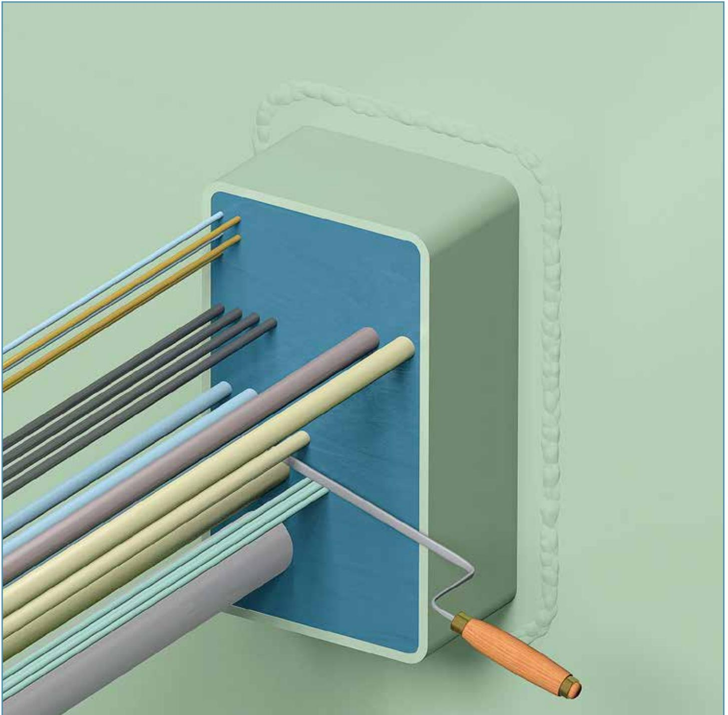
The NOFIRNO® sealant between the cables is pressed down and smoothed by hand or with a spatula or putty knife. A special tool, developed by BEELE Engineering, with a PTFE compression/smoothing part is available. The sealant will not stick to the PTFE.
