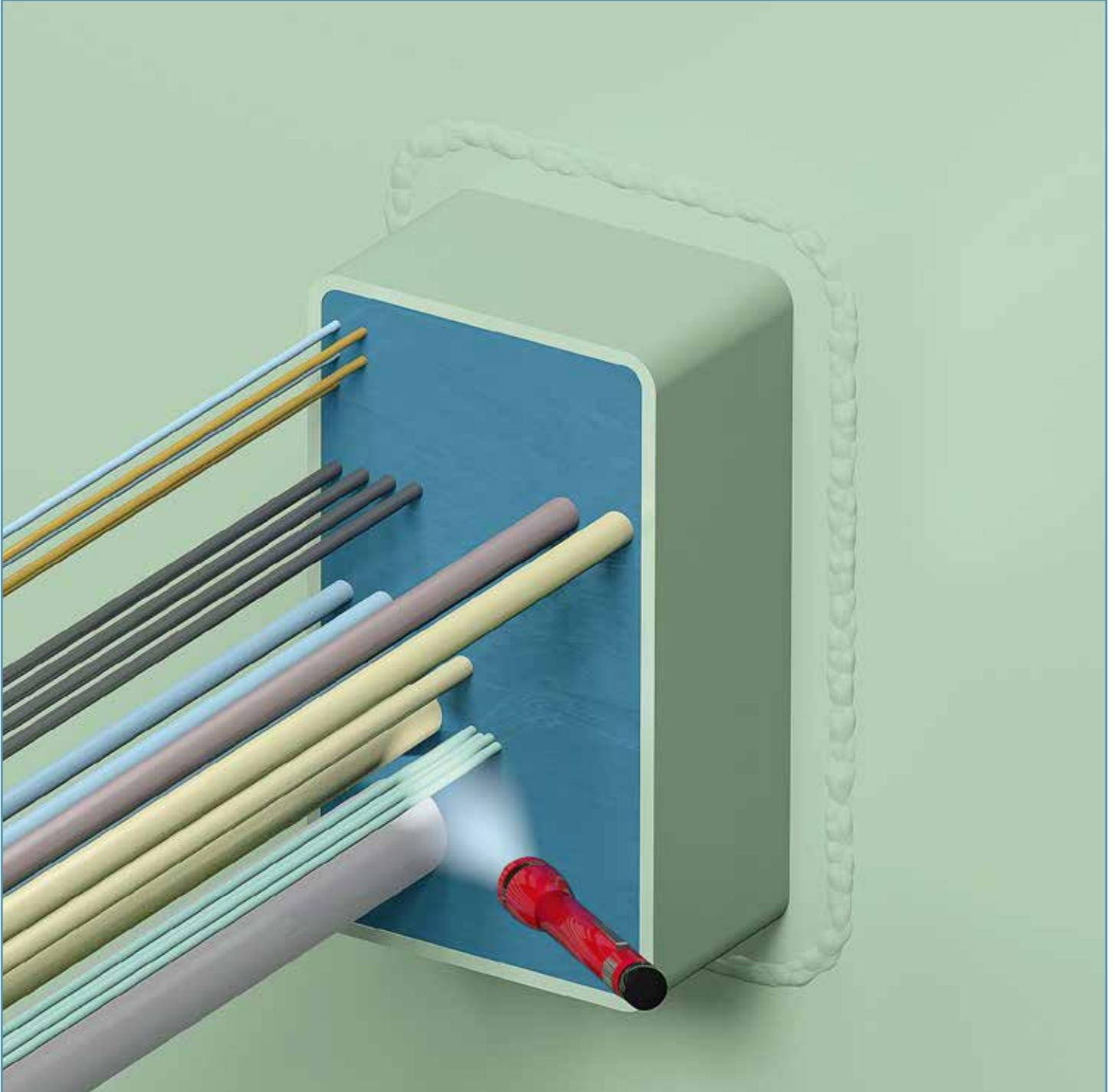
After smoothing is finished, a last check should be taken to ensure sufficient sealant has been applied in between the cables (especially for transits with larger amounts of cables). This is most important for water and gas tight penetrations.
