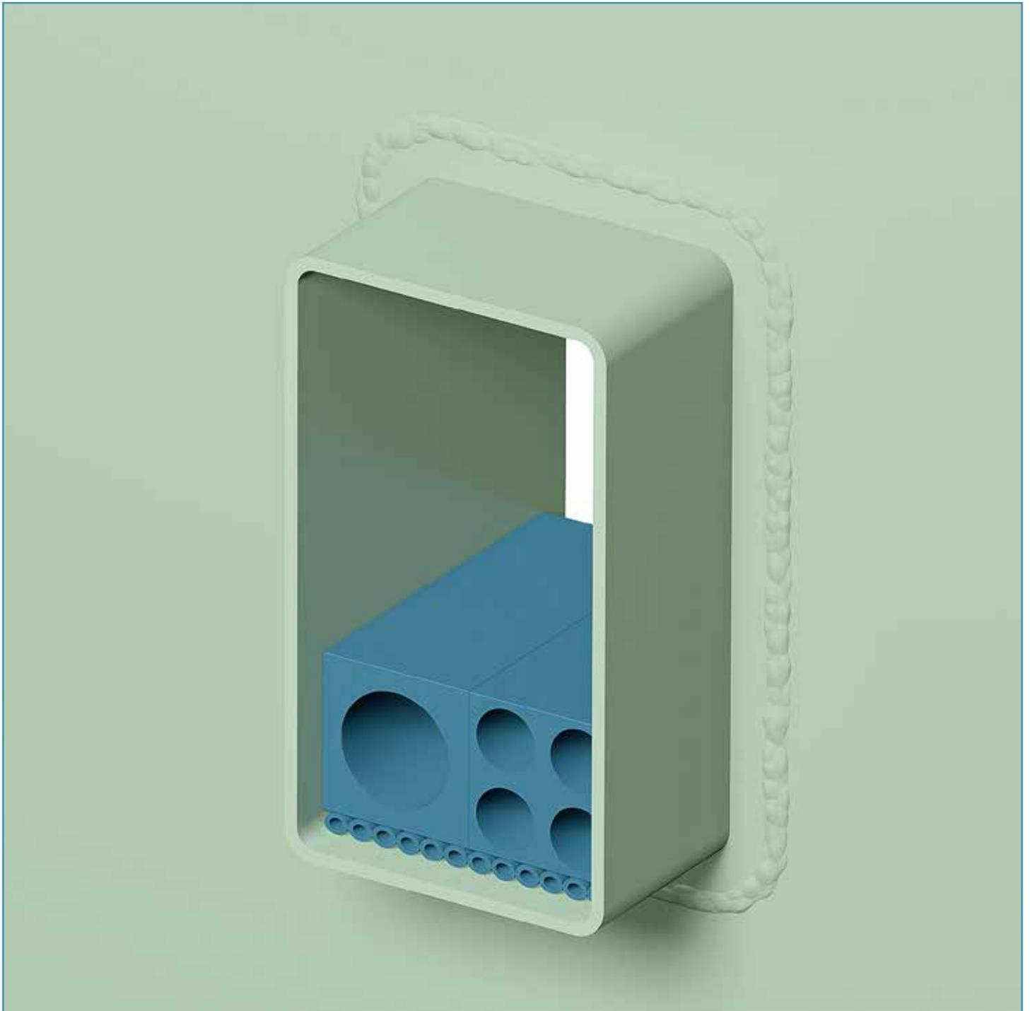
A CONTROFIL® fill plate or a fitting CONTROFIL® multi-sleeve, with a height equal to the bending radii of the corners of the transit frame is placed at the bottom of the frame. This is needed to prevent the blocks from being inserted in the bending radii of the frame.
