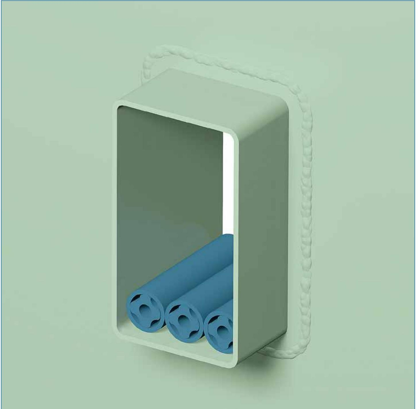
The CONTROFIL® multi-sleeve (MS) type multi-cable transits are specially developed to avoid overfilling of multi-cable transits. Lay-outs on the basis of cable diameters in brochures, include a fair risk that at the end cable diameters at site are totally different. Open transits at site allow for pulling more cables through than planned. Sealing the multi-cable penetration will then be difficult or not possible at all.
