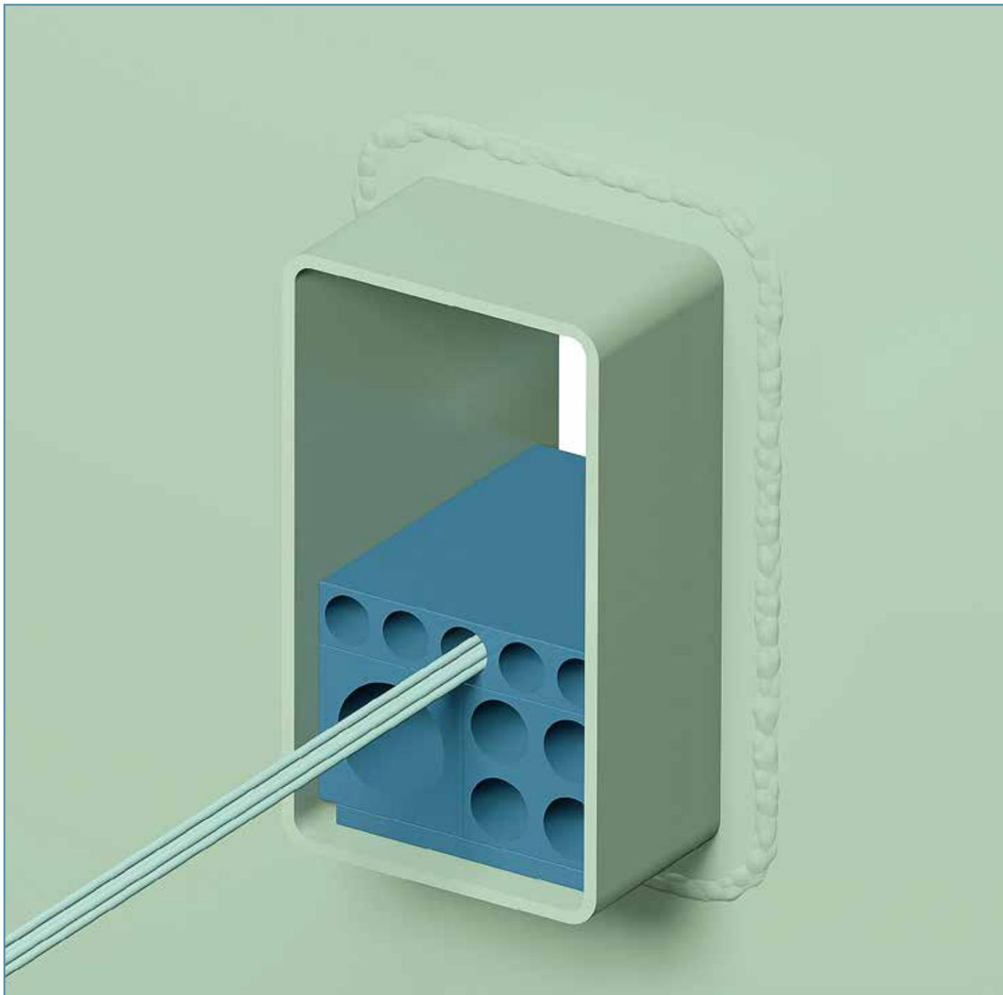
On top of the fill plate/sleeve, CONTROFIL® multi-blocks are stacked. Multi-blocks are 60x60 mm or in a row version with different heights and a width of 120 mm. Available depths of the blocks are 60 mm, 110 mm, 140 mm, 160 mm and 210 mm. The multi-blocks are not used for final sealing of the multi-cable transit; they are a ducting facility. The CONTROFIL® multi-block passage holes allow for ducting one or several cables.
