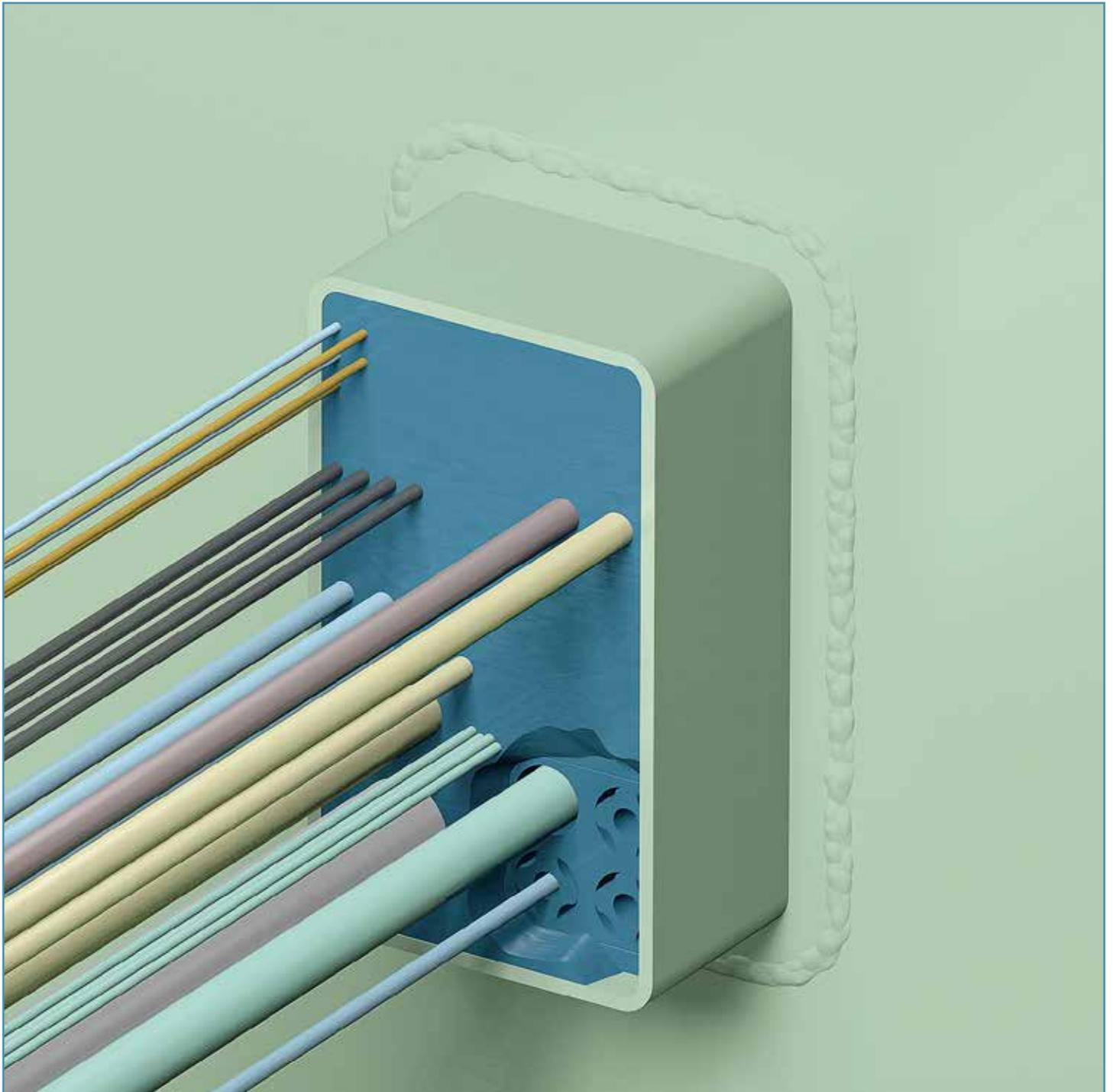
A cable is pulled through the free passage opening of the CONTROFIL® multi-block. For adding cables, there is in fact no more disassembling needed than removing a block filler. No extra costs for the extension of the cable set other than some new sealant to be applied.
