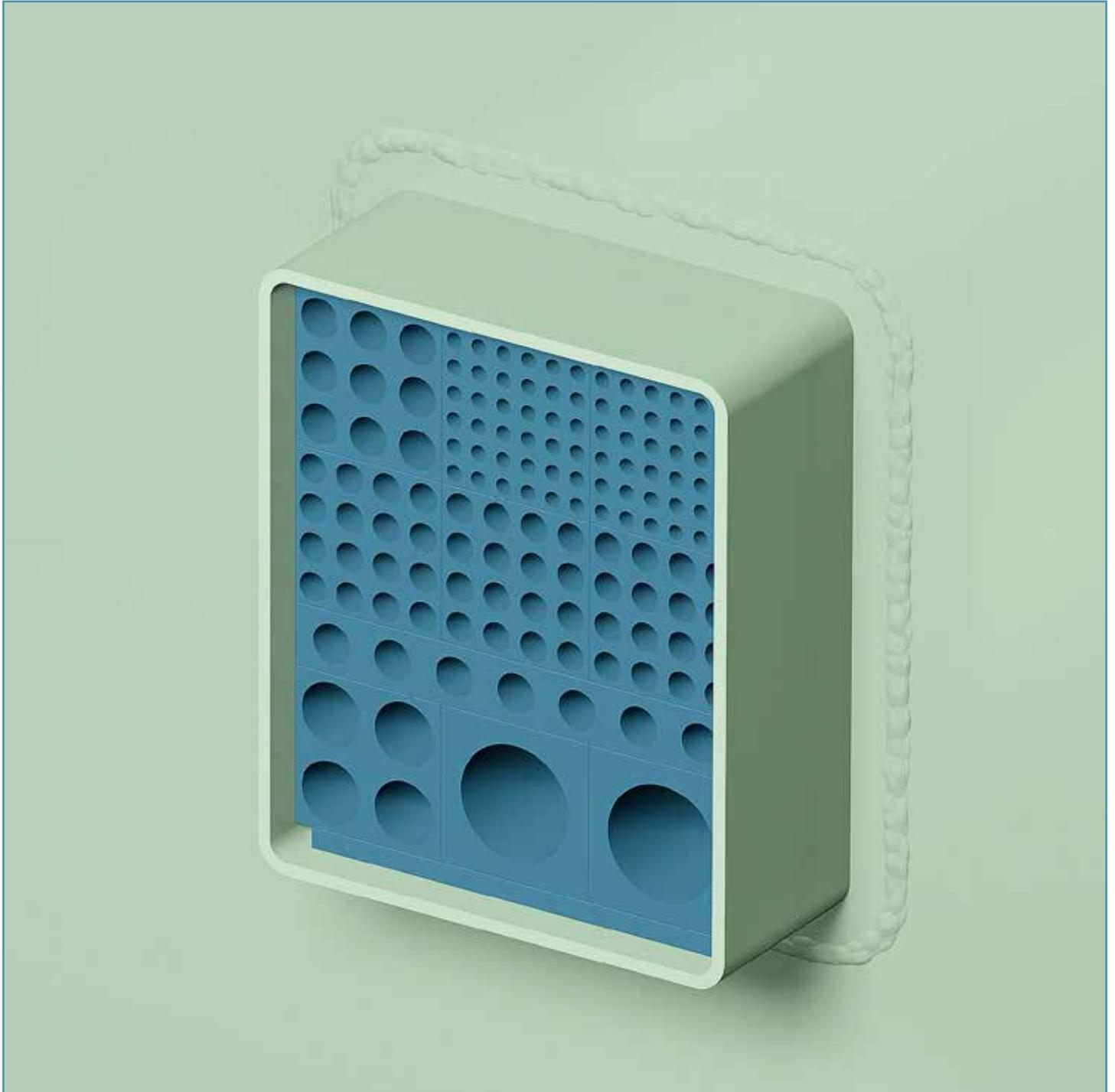
The CONTROFIL® transit frames are available also in sizes 220x180 mm. This means that 3 blocks 60x60 mm can be inserted next to each other. The single row blocks are delivered with a width of 180 mm instead of 120 mm. In this way the configuration for ducting cables in a single transit is substantially extended.
