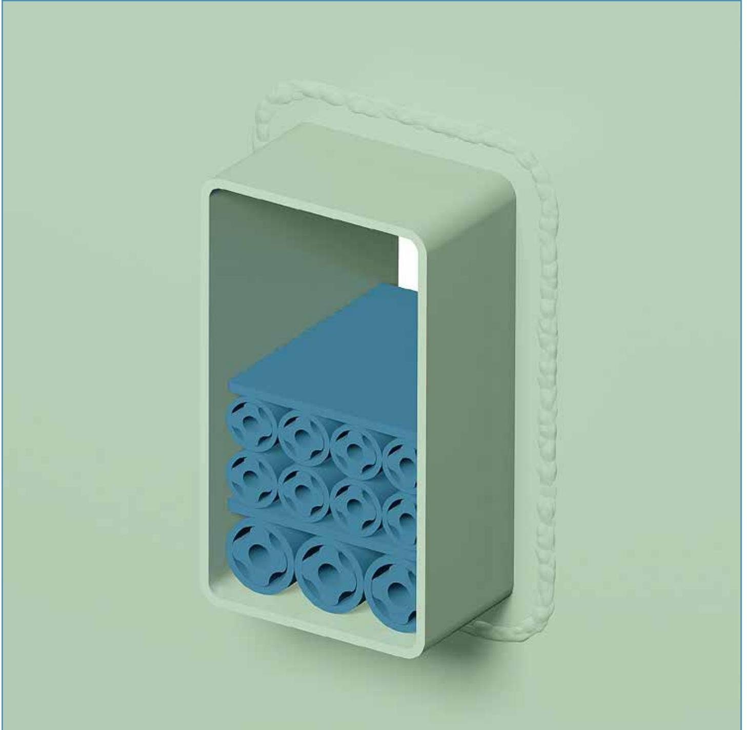
There is no need to place CONTROFIL® separators between rows of identical multi-sleeve types. Another CONTROFIL® separator is placed on top of the set CONTROFIL® multi-sleeves
