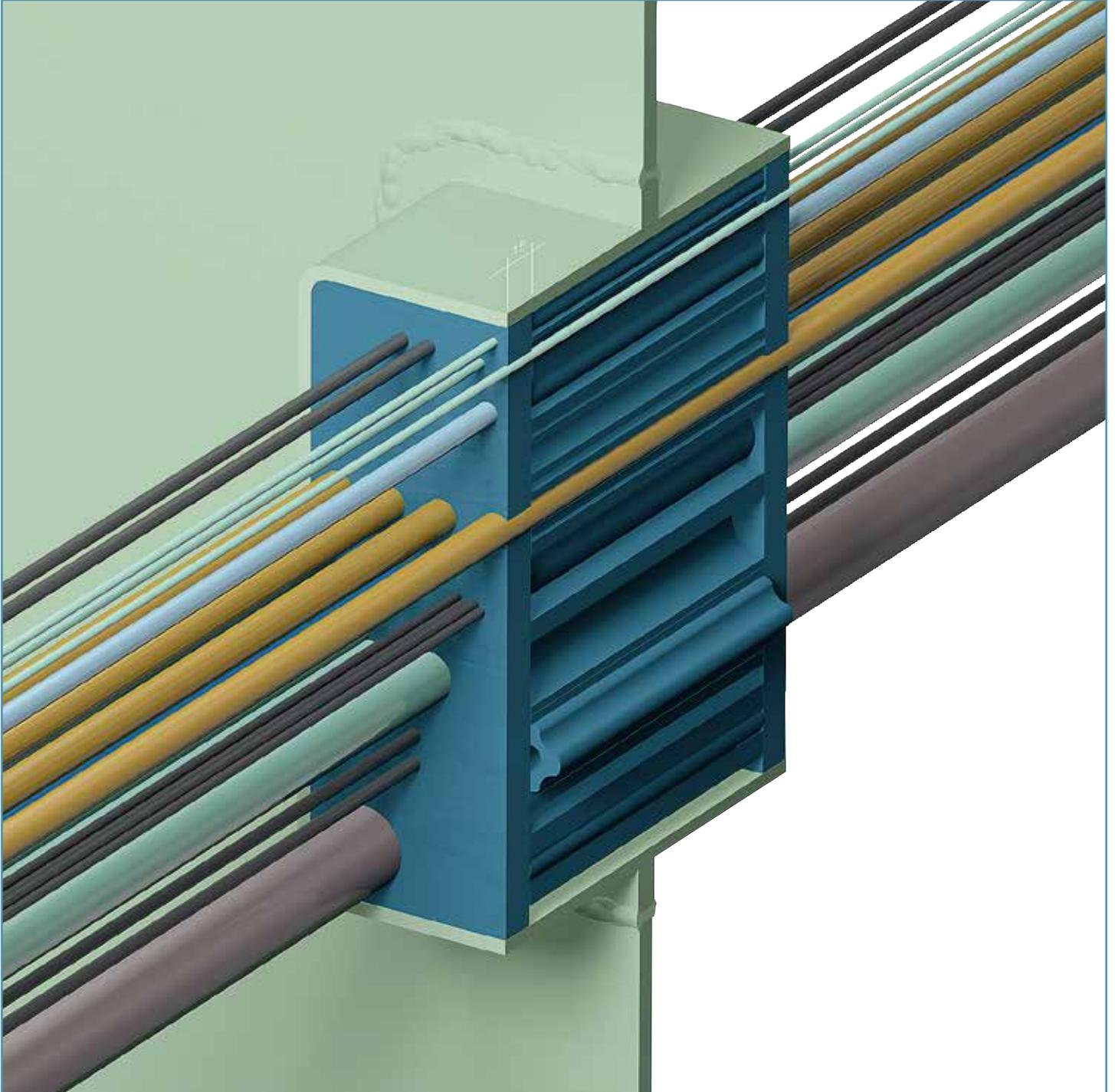
For A-class penetrations (which are insulated), the CONTROFIL® multi-cable transit frame needs to be insulated only at the insulated side of the bulkhead or at the lower side of the deck. No extra insulation needed in front of the penetration and/or in between the cables. Tested with larger amounts LAN data cables (bundled as well) up to CLX high voltage cables up to 3 x 380 mm<sup>2</sup> with an OD of 105 mm. Note: for the larger cable sizes CONTROFIL® cable sleeves and wraps have to be used.
