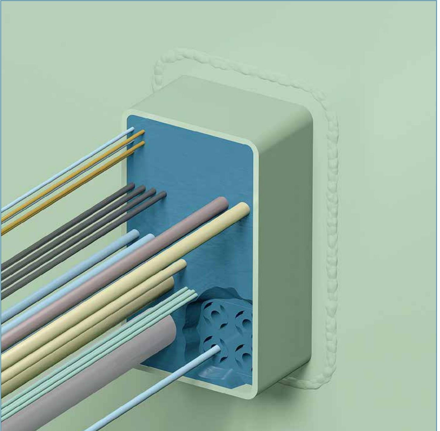
In case a small diameter cable has to be pulled through, the free space around or in the center of a CONTROFIL® block filler can be used. The blocks with smaller passage openings have no filler blocks and the cable can be pulled through the open passage hole.
