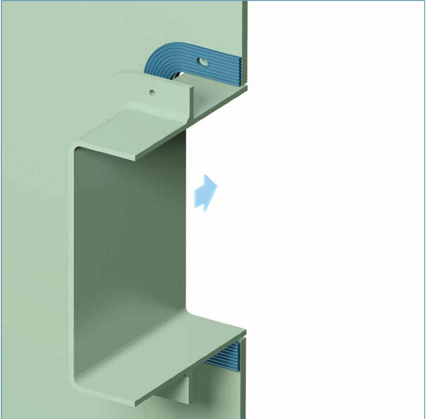
The CONTROFIL® flanged transit frames are bolted against the partition. A firesafe NOFIRNO® gasket has to be applied between the flange of the transit frame and the partition. The gaskets have a designed profiling to exclude the need for excessive compression (6-10 Nm is sufficient). The reduced forces on the profiled rubber makes the usual need for retightening from time to time a thing of the past.
