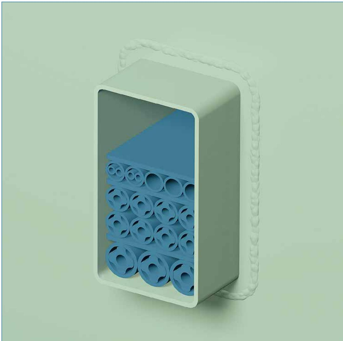
One or several CONTROFIL® cable or filler sleeves can also be placed in the non-used openings. CONTROFIL® multi-sleeves are available with different heights and a width of 120 mm. Available lengths of the sleeves are 60 mm, 110 mm, 140 mm, 160 mm and 210 mm. The multi-sleeves are not used for final sealing of the multi-cable transit; they are a ducting facility.
