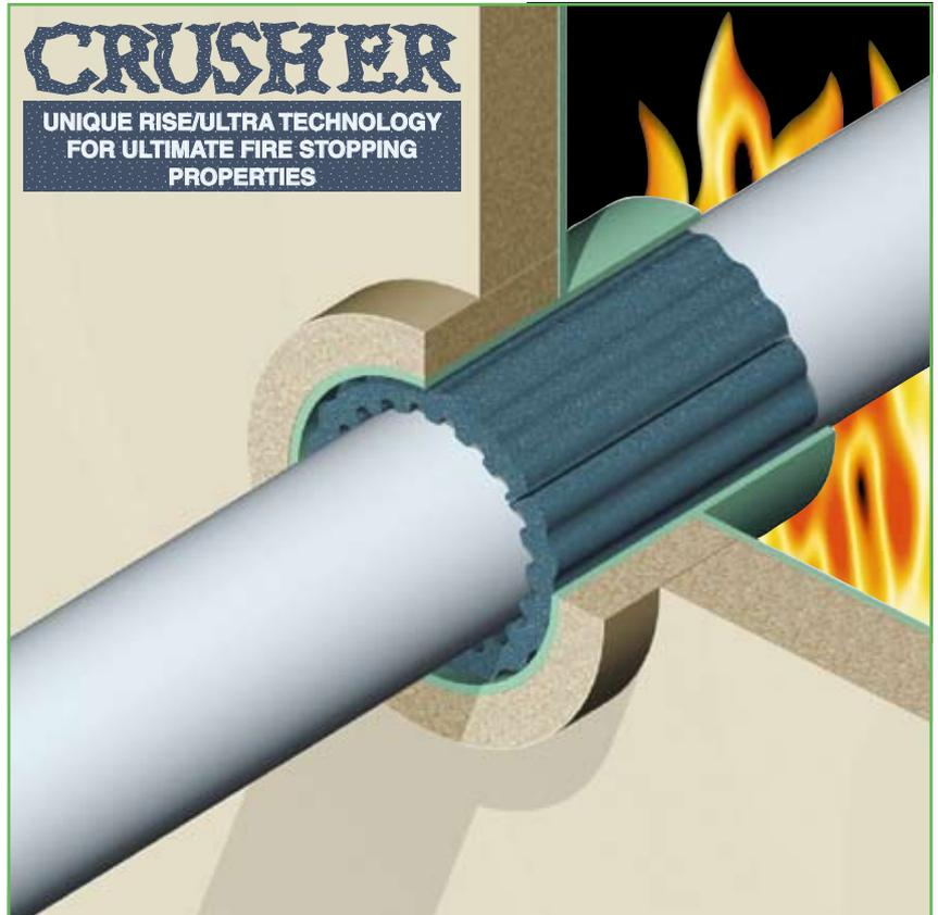
A fair amount of fire tests have shown that the depth of the conduit opening can be minimum 180 mm for plastic pipes up to 140 mm OD, and 200 mm above 140 mm OD. Fire tests have shown that the formed adhesive mass prevents shrinkage of the expanded rubber during and after fire exposure.
