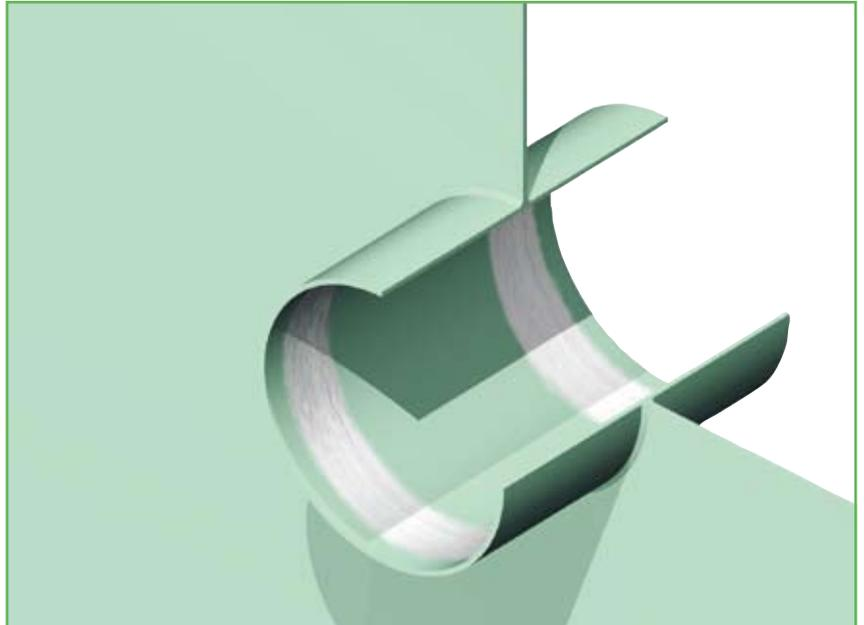
The NOFIRNO®-EMC system based on 2 layers of 40 mm CONDUCTON® flexible rubber. Attenuation: 52->100 dB.
