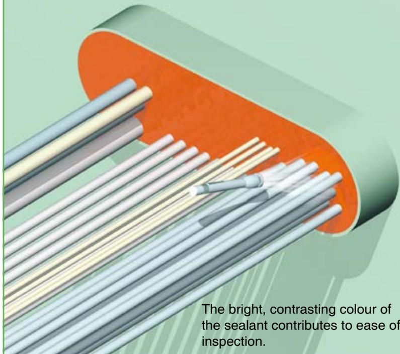
The bright, contrasting colour of the sealant contributes to ease of inspection.
