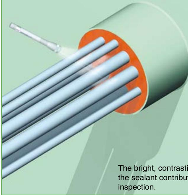
The bright, contrasting colour of the sealant contributes to ease of inspection.
