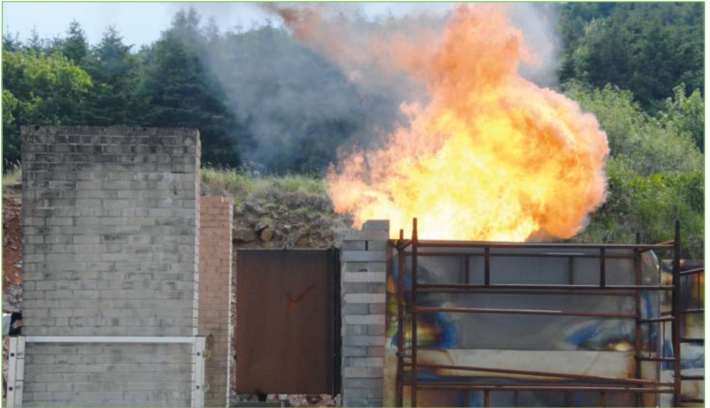
JET FIRE TEST ACCORDING TO ISO 22899-1:2007 AND ISO/CD 22899-2
