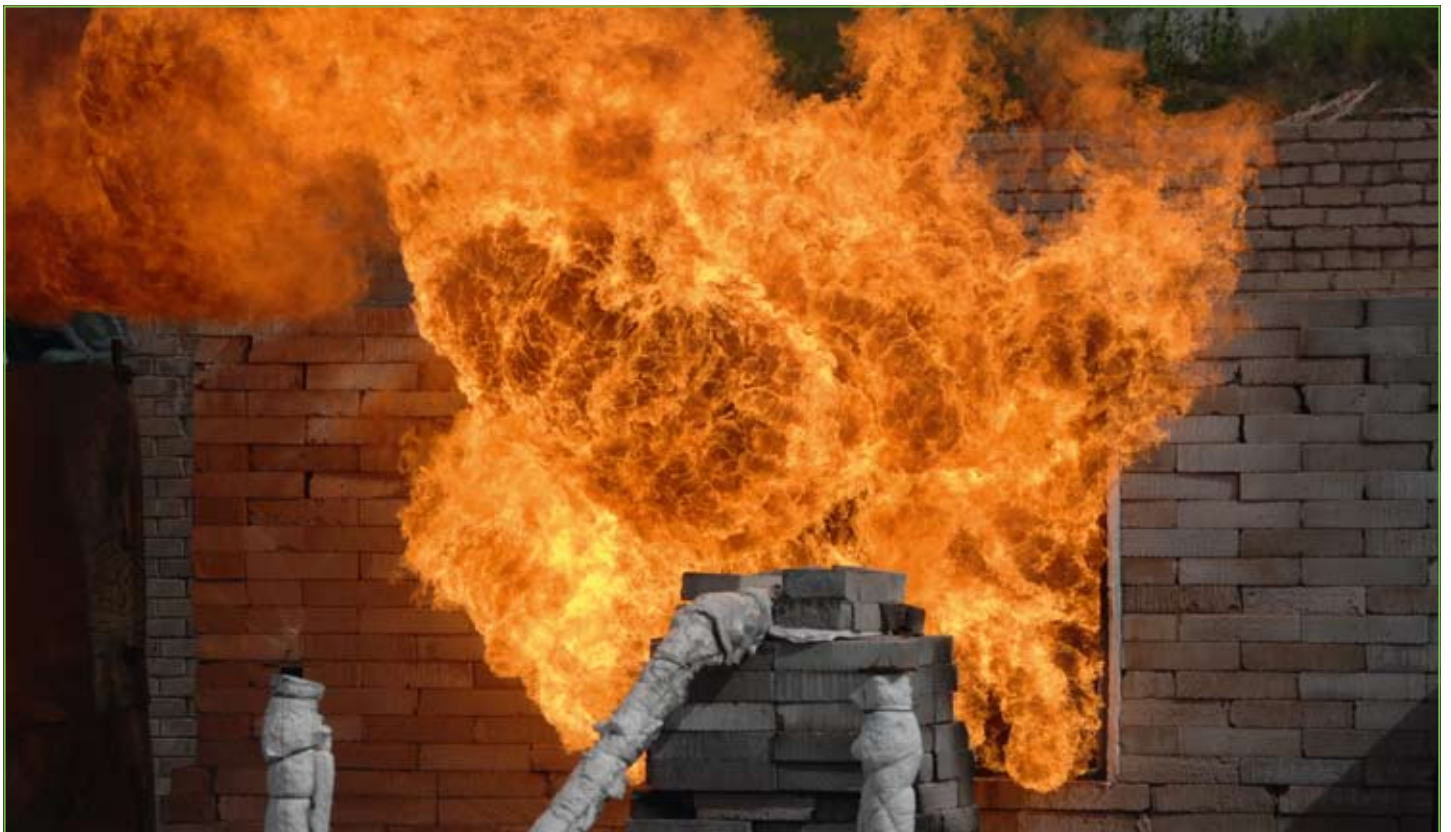
JET FIRE TEST ACCORDING TO ISO 22899-1:2007 AND ISO/CD 22899-2
