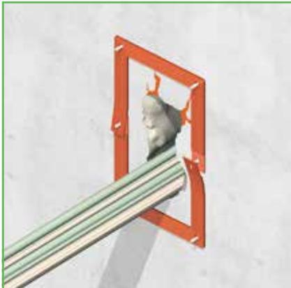
4) After drilling the attachment holes and positioning the anchoring bolts, place the NOFIRNO® gasket parts over the anchoring bolts against the wall.
