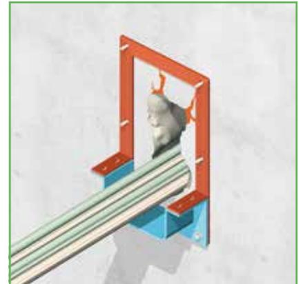
6) Place the NOFIRNO® gaskets on the connector flanges of the CSD® split flanged frame.
