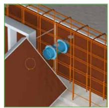
6) The formwork element is then removed so that the CSD<sup>®</sup> fixation piece can be affixed.
