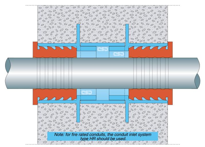
Optimized gas and water tightness is obtained by applying the SLIPSIL<sup>®</sup> sealing plugs in the CSD<sup>®</sup> embedded conduit inlet system or in the CSD<sup>®</sup> flanged conduit sleeves.
