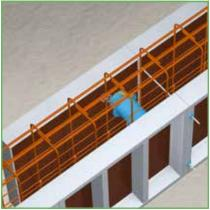
5) The formwork element is provisionally positioned so that the position of the CSD<sup>®</sup> fixation piece to be fitted can be marked off.
