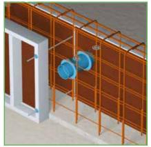
4) The CSD<sup>®</sup> embedded conduit inlet system must also be affixed to the formwork element on the other side using a fixation piece in order to obtain sufficient stability during the pouring of the concrete.
