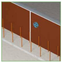
1) After marking off on the formwork, CSD<sup>®</sup> fixation pieces suitable for CSD<sup>®</sup> conduit inlets are fastened by means of nails or screws.
