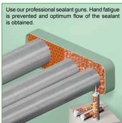
14) When working on larger conduits, the sealant should be applied in two or more parts. Due to the fast curing of the top layer of the sealant, the amount of sealant should not be more than can be finished within 10 minutes.
