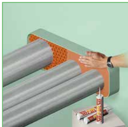
16) The surface can be smoothed by hand. Wet the hands thoroughly with soap and water to avoid the NOFIRNO® sticking to the hands. A very neat surface is the result. Prevent soap water to be applied on the sealant surface on which the next sealant will be applied.
