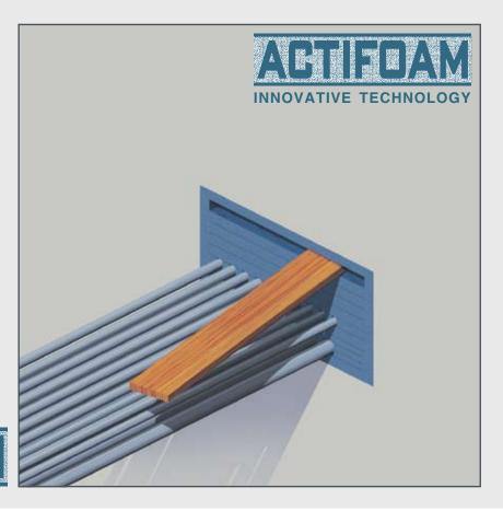
19) The finished ACTIFOAM<sup>®</sup> multi-cable penetration. Officially fire tested according to EN 1366-3:2004 and classified according to EN 13501-2:2003 (NEN 6069) for two hours in an aerated concrete wall 150 mm thick.
