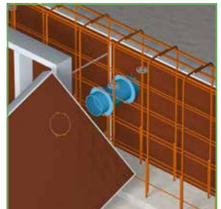
6) The formwork element is then removed so that the CSD® fixation piece can be affixed.
