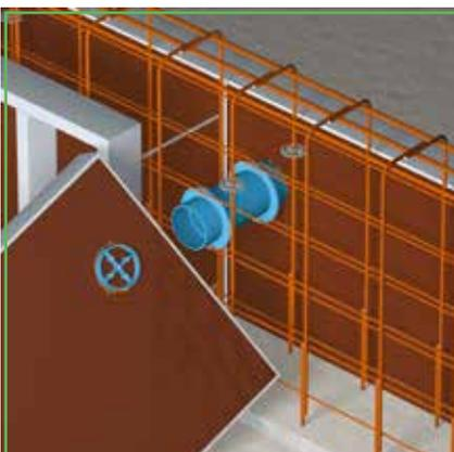
7) The CSD® fixation pieces are made to be for clamping fit for fixation in the CSD® conduit inlets for reasons of stability but also to prevent concrete running into the conduit inlets.
