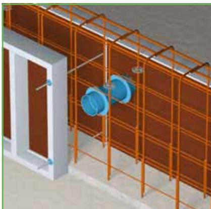
4) The CSD® embedded conduit inlet system must also be affixed to the formwork element on the other side using a fixation piece in order to obtain sufficient stability during the pouring of the concrete.
