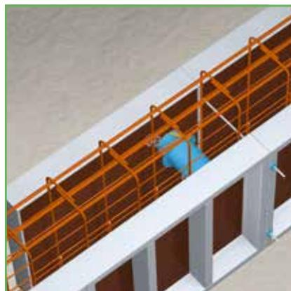
5) The formwork element is provisionally positioned so that the position of the CSD® fixation piece to be fitted can be marked off.
